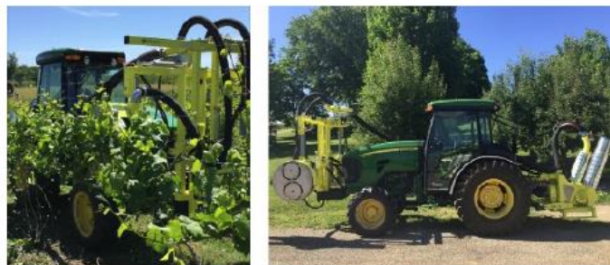
Figure 2.5 Left: whole view of the leaf remover, Right: the machine shattering leaf between two rows.
